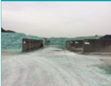
Outside storage of colour segregated cullet ready to be used at a float glass plant
